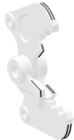
Cracker Wear Plate Location FIGURE 44
