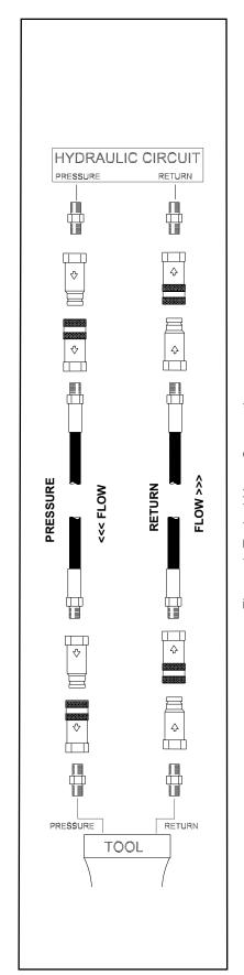
Figure 1. Typical Hose Connections
