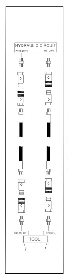
Figure 1. Typical Hose Connections
