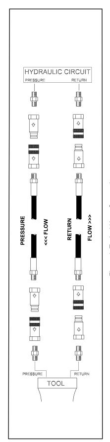
Figure 1. Typical Hose Connections
