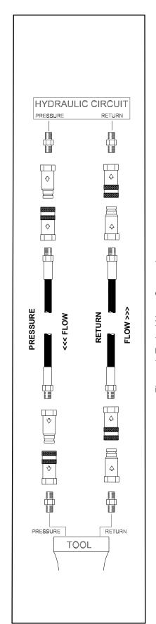
Figure 1. Typical Hose Connections
