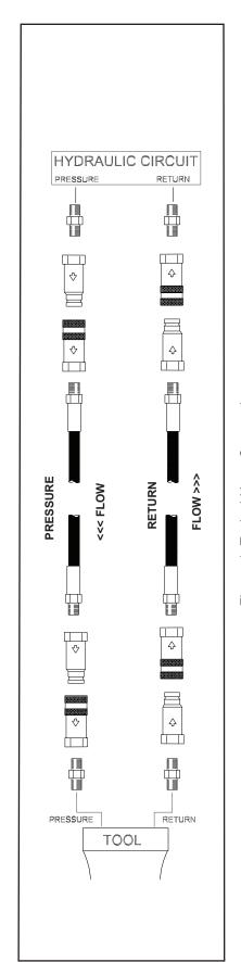
Figure 1. Typical Hose Connections
