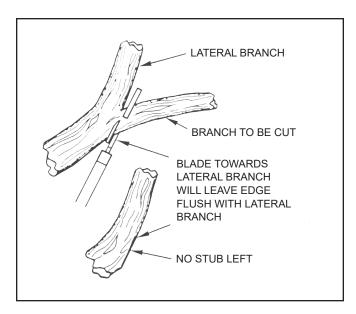
Figure 2. Example of Lateral Branch Cut
