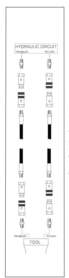
Figure 1. Typical Hose Connections
