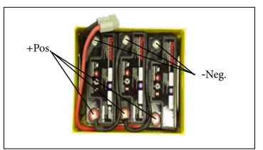
Figure 1: Battery cable and terminals
