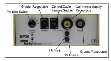
Figure 2: EP30 Connections
