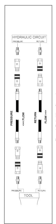
Figure 1. Typical Hose Connections
