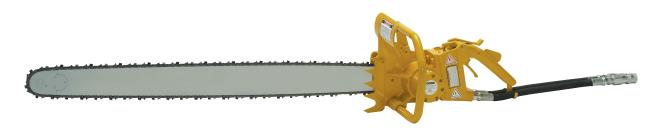
The **CS11** is an extreme duty hydraulic powered chain saw for cutting all types of wood structures underwater - including bridge pilings, pier and dock timbers. It's robust design and high torque gear motor provides divers instant chain speed to cut through the toughest timbers with ease. The power to weight ratio is significantly higher than any other wood cutting chain saw and is available with bar lengths up to 42" (107 cm). Painted hi-visibility yellow.
