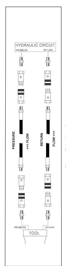
Figure 1. Typical Hose Connections
