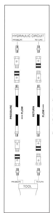
Figure 1. Typical Hose Connections
